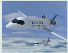
programme aiming to develop a liquid hydrogen propulsion system for subregional aircraft that could be scaled up to larger aircraft. Liquid hydrogen is being converted to electricity within a fuel cell system. This electricity efficiently powers the aircraft, eliminating carbon emissions and creating a new generation of clean air travel.
